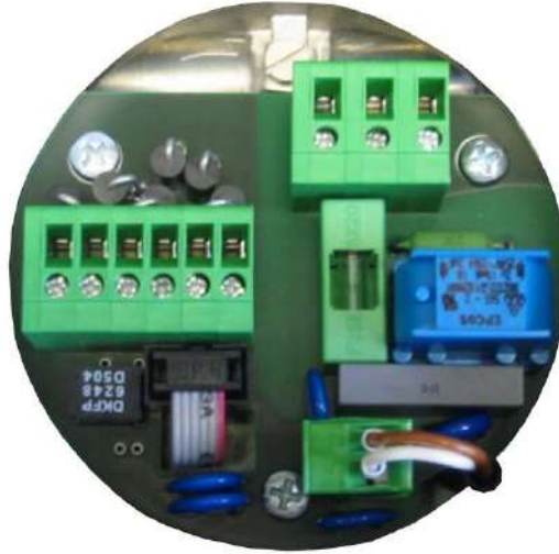
Fig. 31 - CH1.10 process terminals
