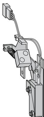
If MCR switch is built in the breaker and the dial for INST/MCR on Main setting module is set to any MCR position, MCR function is operative.
