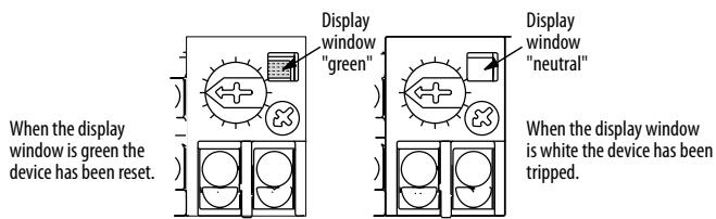
When the display window is green the device has been reset.
