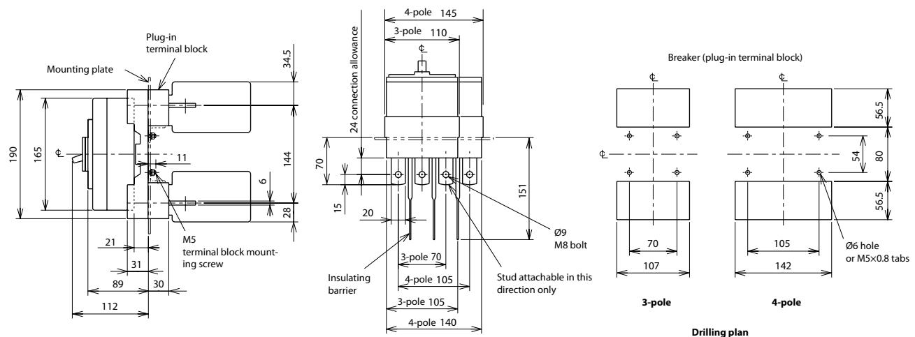
Remark: 1. Two-pole models are three-pole models with the central pole removed.
