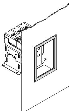
The door frame improves the appearance, after cutting out the panel door to install the breaker. Details on request.
