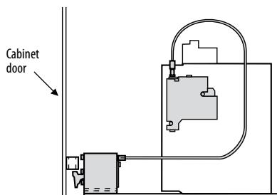
This mechanical interlock device makes it impossible to open the panel door unless the circuit breaker is not switched off.
