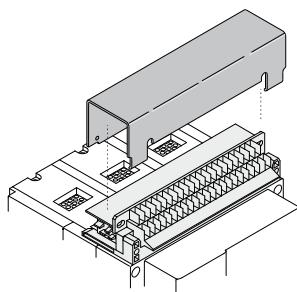
The terminal cover is a transparent cover for safety finger protection of control terminals. The terminal cover prevents from careless touching to the live control terminals. The TTC-F-W is included within the delivery of a fixed type AE-SW as standard.
