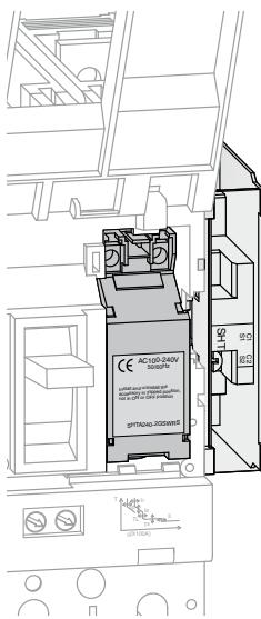
Figure shows Lead-wire terminal block type (SLT).
