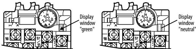
When the green of the display lever can be seen, the device has been reset.
