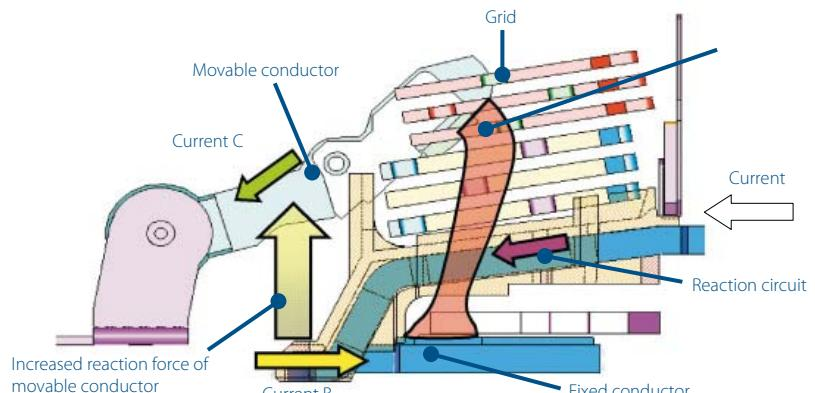
Expanded ISTAC breaking technology
