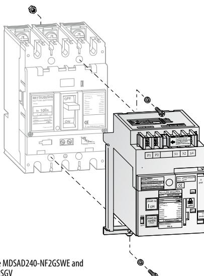
Spring-charged type MDSAD240-NF2GSWE and breaker type NF250-SGV
