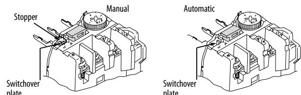
Switching from manual to automatic: Break the stopper off and then, slide the switchover plate to the right (to position "A") to immobilize the reset bar.
