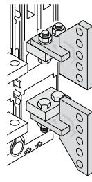
Vertical terminal adapters allow you to turn power connection by 90°.
