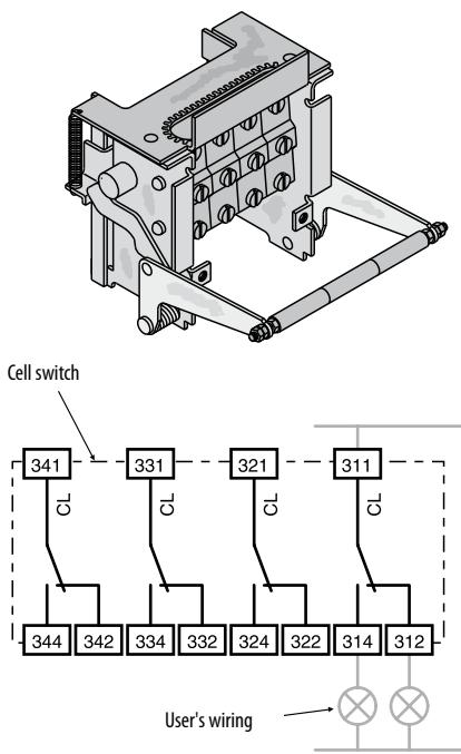
The cell switches can be set for all the relevant positions, i.e. connected, test and disconnected.
