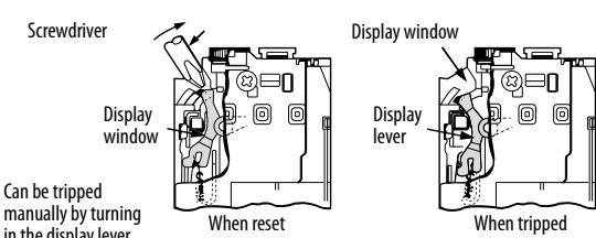
Can be tripped manually by turning in the display lever.
