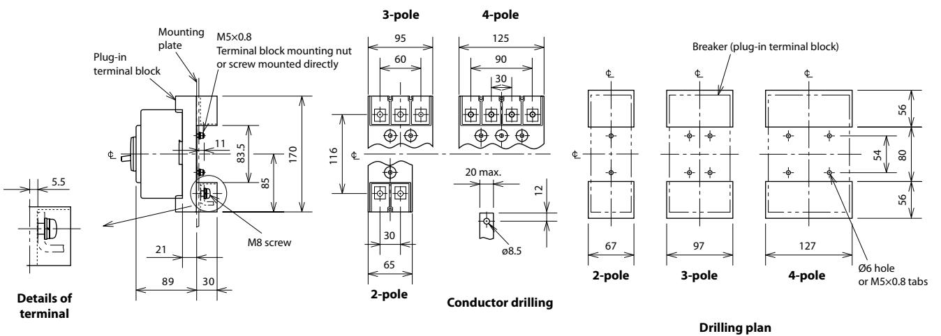
**Remarks:** 1. The two-pole models of NF125-HV are three-pole models with the central pole removed.
