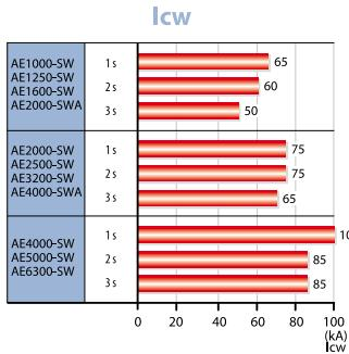
Rated short circuit breaking capacity I<sub>cu</sub> = I<sub>cs</sub>
