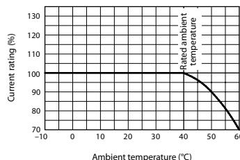
The rated current does not have thermal characteristics. Reduce the current as shown in the curve on the left chart if the ambient temperature exceeds 40°C.
