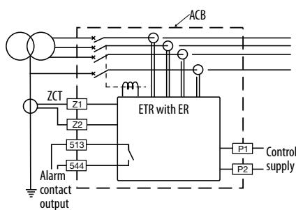
This option is used to detect several amperes of earth leakage when used in combination with an electronic trip relay that has the earth leakage tripping (ER) option.
