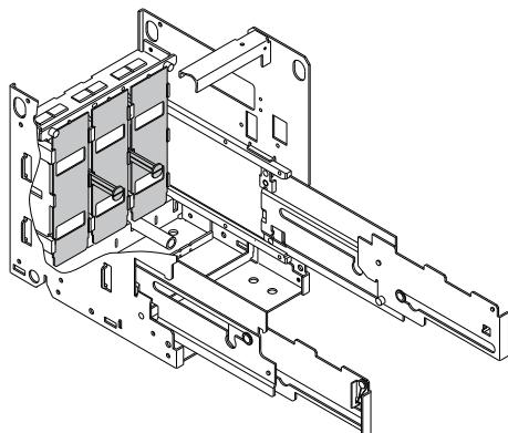
The safety shutters cover the main conductors of the cradle side (supply and load side) automatically when the circuit breaker is drawn out.
