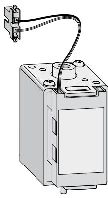
The closing coil is a device to close the breaker by remote control. Only one closing signal (about 100 msec.) is sent even when the closing coil supply is maintained ON.
