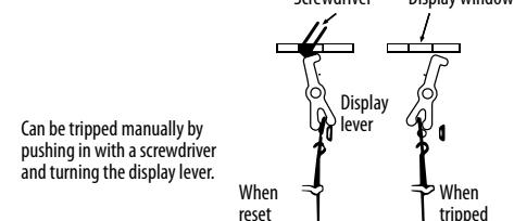
Can be tripped manually by pushing in with a screwdriver and turning the display lever.
