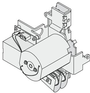
In addition to manual operation, the closing spring can be charged automatically by an electric motor every time the breaker is closed (ON charging method).
