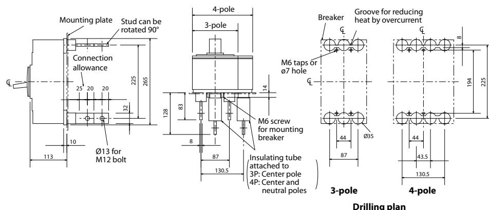
Boring dimensions for rear connection type barriers (3-pole)
