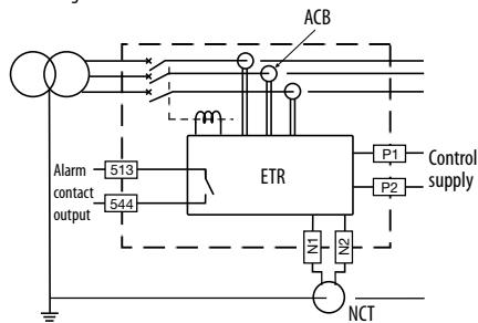
The neutral CT is used for ground fault protection when a 3 pole breaker is used on a 3 phase 4 wire system.
