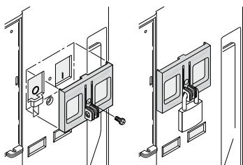
This mechanical device can be locked with a padlock or a seal (both is not included in the package) to protect the push buttons of the breaker unit against inadvertent ON/OFF operation.
