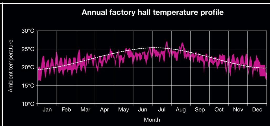
Rittal specifies the SEER to indicate the actual efficiency of a cooling unit, since a precise calculation must also consider the seasonal temperature variation. The standard point for determining the EER does not make allowance for actual fluctuations in hall temperatures.
